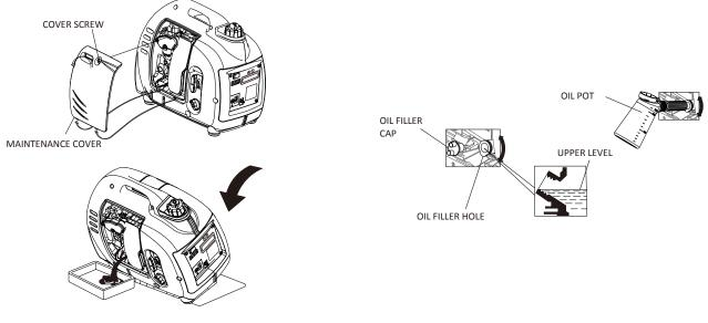
HY1000Si Oil Capacity: 0.25L HY2000Si Oil Capacity: 0.40L
