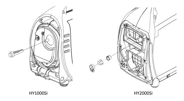
8.4.3 Remove carbon deposits of the spark arrester using a wire brush. If the spark arrester is worn, replace it.
