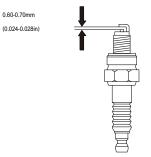
8.3.6 Measure the spark plug gap with a feeler gauge. The normal value: 0.6-0.7mm (0.024-0.028in). Adjust the gap by bending the electrode carefully.
