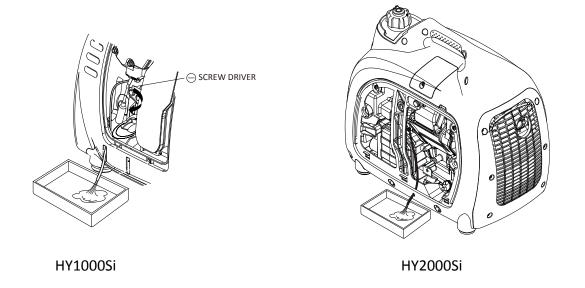
c. Take off the spark plug cap, pull the recoil starter grip three or four times, discharge the petrol from the fuel pump and fuel lines.
