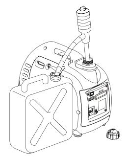
b. Turn the engine switch to "ON" position, and loosen the carburetor float bowl drain screw to discharge from inside of carburetor float bowl.
