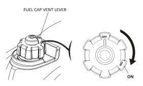
5.2 Turn the engine switch to the "ON" position.
