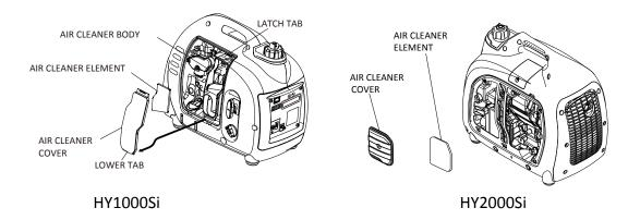
8.2.3 Take out the air cleaner element, and clean it with a non-flammable or high flash point solvent, then dry it.
