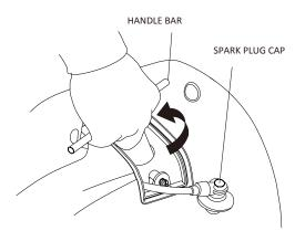
8.3.4 Take off the spark plug with the spark plug spanner.
